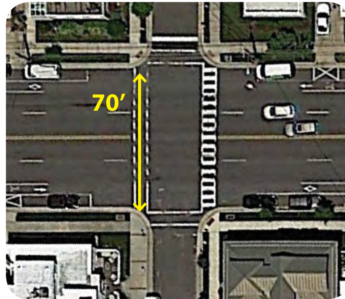
TYPICAL UN-SIGNALIZED INTERSECTION
